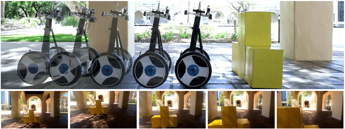
Fig. 4. Images from the experiment using the MR-BS-OP controller. The Segway is piloted towards a wall of yellow boxes and the controller ensures that it remains safe, i.e. that it does not crash into the boxes. (Top) Time lapse of the Segway trajectory. (Bottom) Camera images taken from the perspective of the Segway throughout the experiment. The images are displayed in chronological order from left to right. A video can be found at [25].
